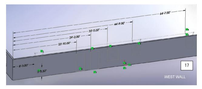
18. After we do our Extrude Cut features into the exterior walls and start adding some of our part models, the Mercy Building assembly should resemble the image below.
