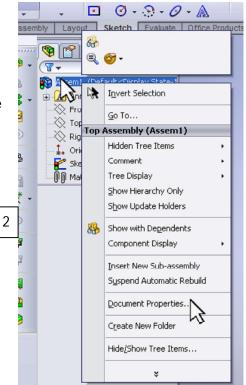
3. Next choose "Units", then to the right of the menu choose "Custom" just below that click on the down arrow for the length then select "feet & inches". Click on the "OK" button on the bottom of the dialog box. When you go back to your model area the sketch should have the appropriate dimensions displayed as entered in the previous sketch.
