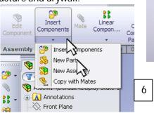
"Assembly" tab. Select the pull down arrow on the "Insert Component" button. Then select the "New Part" option. SolidWorks will now be asking you for the plane that you want to reference the Front Plane of the New Part to (the cursor will have a green check mark next to it). Choose the Front Plane of the assembly in the Feature Manager.
