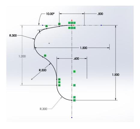
Front base sketch details, before the mirror command, grey scale dimensions are "driven" dimensions and are derived from other sketch geometry.
